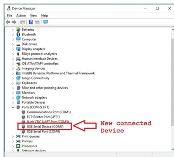
Communicate via this Serial device (EX. By TeraTerm @115200,N81).
